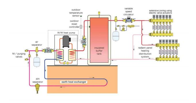
The system needs thermal mass. That mass has been added as a well-insulated buffer tank. It also should have an expansion tank and air eliminator on the earth loop. I also like to specify a low-velocity zone dirt separator within the earth, as shown on the Fix drawing.
